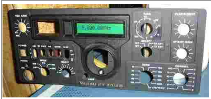
Front face showing DFD installation
