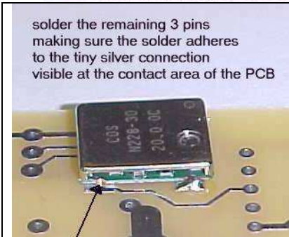
flow a thin layer of solder on pad 1
